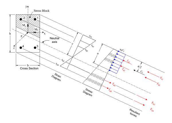
Figure 2-1 Analysis of Reinforced Section
