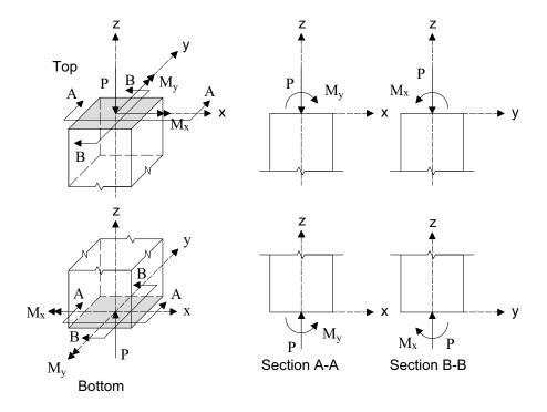
Figure 2-4 Positive axial force and bending moments (internal forces)
