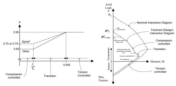
\*Spiral sections in compression controlled zone:  $\phi$  = 0.75 per ACI 318-14/11/08 and  $\phi$  = 0.70 per ACI 318-05/02
