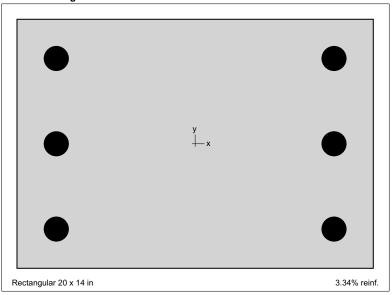
Figure 1: Column section
