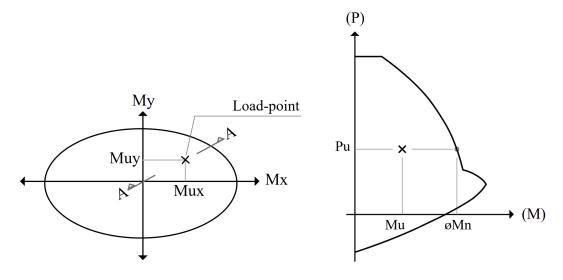
Section A-A (P-M Diagram)
