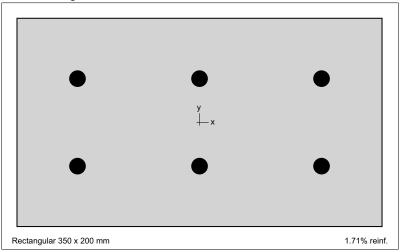
Figure 1: Column section
