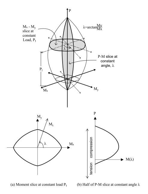
Figure 2-7 Interaction Surface for Combined Axial Load and Biaxial Bending
