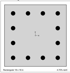
Figure 1: Column section
